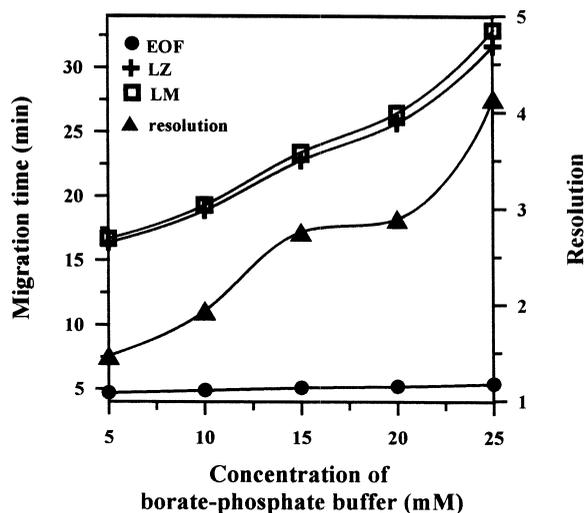
Fig. 2. Influence of the concentration of borate–phosphate buffer on migration times and resolution (● EOF, □ LM, + LZ and ▲ resolution). Background electrolyte: 50 mM SDS, 10% acetonitrile, 25 °C and 20 kV.
