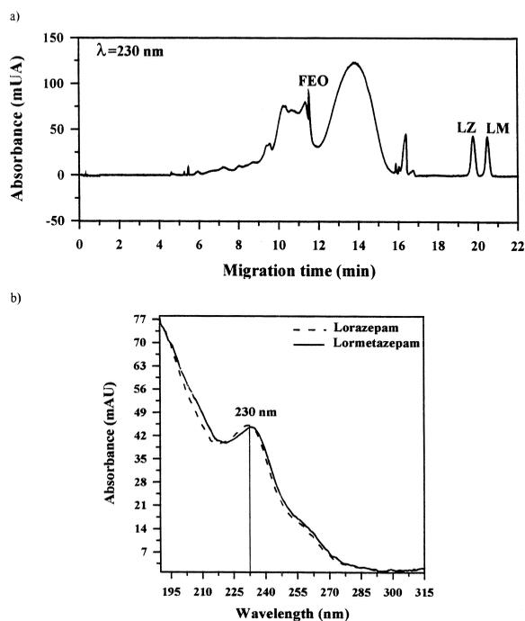
Fig. 4. (a) An electropherogram obtained under the selected conditions (15 mM borate–phosphate buffer, pH 8, 30 mM SDS, 15% methanol, 25 kV and 30 °C); (b) spectra of lormetazepam and lorazepam.
