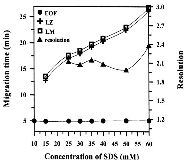
Fig. 3. Influence of the concentration of SDS on the migration times and resolution (● EOF, □ LM, + LZ and ▲ resolution). Background electrolyte: 15 mM borate–phosphate buffer, 10% acetonitrile, 25 °C and 20 kV.
